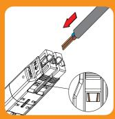
Orientate and align pre-cut cable and insert into appropriate cable entry point. Each wire should guide itself into the correct terminal. Push cable until there is resistance.
