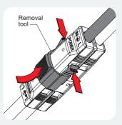
Mount removal tool. Place thumb on thumb grip and using other hand, squeeze side arms so they locate beneath the snaps.
