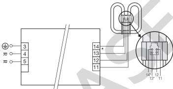
\* leads 13, 14 max. 1.0 m (< 100 pF) leads 11, 12 max. 2.0 m (< 200 pF) For luminaires of protection class I: Earthing via ECG casing or earth terminal (according to IEC 60598) For luminaires of protection class II: No earthing required
